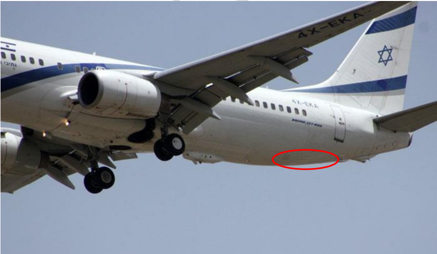
A C-MUSIC system has been installed on one of El-Al Boeing 800-737 aircrafts. Photo: Elbit Systems
