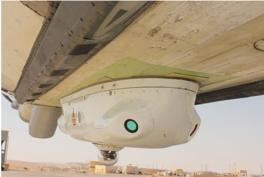
A C-MUSIC system has been tested on one of the Israeli Air Force Boeing 707 flying tanker. Photo: IMOD
